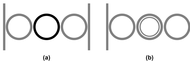
Fig. 1 Two approaches to frequency trimming at fabrication. (a) When a maskless lithography technique is used such as scanning-electron-beam lithography, the exposure dose of a given resonator can be altered to introduce slight dimensional changes resulting in precise resonant frequency trimming. (b) When a mask-based lithography is employed such as optical projection lithography or nano-imprint lithography, a non-resonant dielectric structure evanescently coupled to the resonant mode is introduced to precisely modify the resonant frequency of the micro-cavity.
