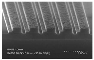
Fig. 3. Angled cross section micrograph showing an example vertical grating coupler fabricated by full and partial thickness polysilicon etches. Note etch profile and surface roughness.
