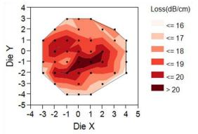
Fig. 4. Polysilicon waveguide bulk loss at 1280 nm measured on a single end-of-line 200 mm wafer. The attenuation ranged from 15 dB/cm to 21 dB/cm with a sample size of 40.
