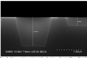
Fig. 2. Cross section micrograph showing adjacent Deep Trench Isolation (DTI) and Shallow Trench Isolation (STI). DTI enables fabrication of FEOL waveguides without undue coupling to the substrate, while the standard STI is used for the standard CMOS.
