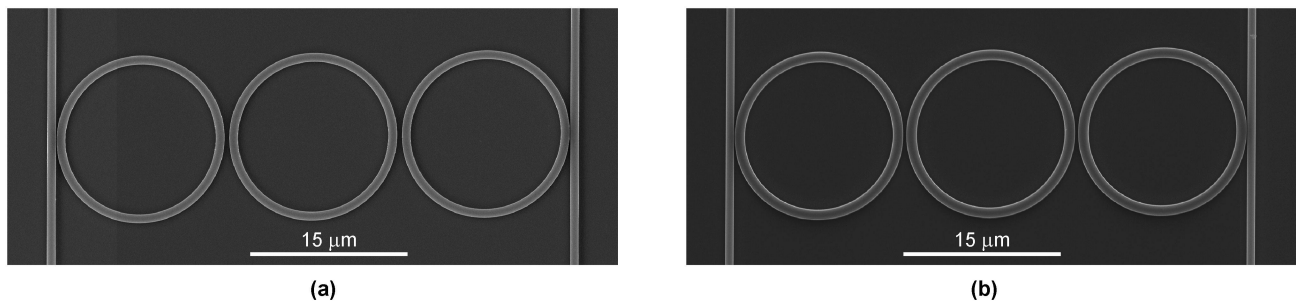
Fig. 3 Electron micrographs of fabricated filters with (a) symmetric coupler design and (b) with asymmetric coupler design.
