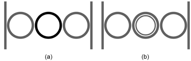
Fig. 5. Frequency-matching strategies. (a) SEBL dose of the middle ring is increased to precisely widen the middle-ring waveguide. (b) Secondary nonresonant ring is introduced at the center of the middle ring to increase the effective index of the middle ring waveguide. Both methods lower the resonant frequency of the middle ring to match it to the outer rings. (a) is particularly useful if a maskless lithography technique, such as SEBL, is used and can be applied in either mask fabrication or direct device writing. (b) is particularly useful for photolithography or nanoimprint lithography when little control is exerted on the mask-manufacturing process.
